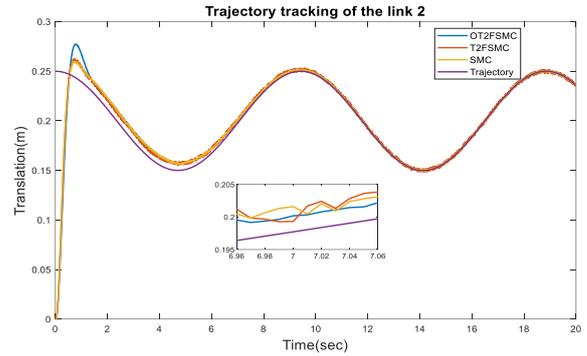
Fig. 13. Trajectory tracking performance of the link 2
