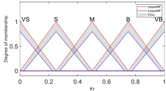
Fig. 6. The membership function of reaching gain
