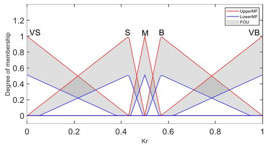
Fig. 11. The optimal membership function of reaching gain
