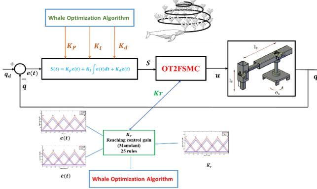
Fig. 7. The Optimal type 2 fuzzy sliding mode control structure
