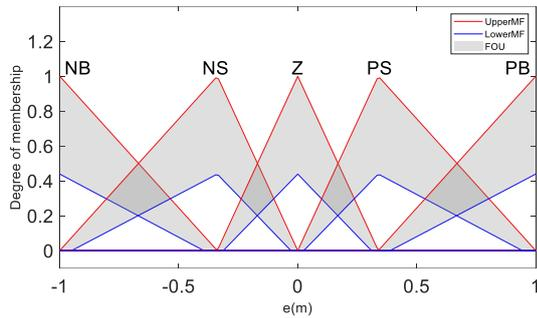
Fig. 9. The optimal membership function of error
