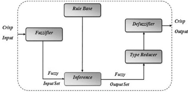
Fig. 2. Structure described the interval type-2 fuzzy logic controller [16]
