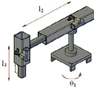
Fig. 1. Cylindrical robotic arm [13]
