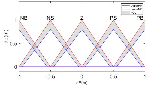
Fig. 5. The membership function of rate of error
