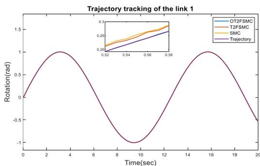
Fig. 12. Trajectory tracking performance of the link 1
