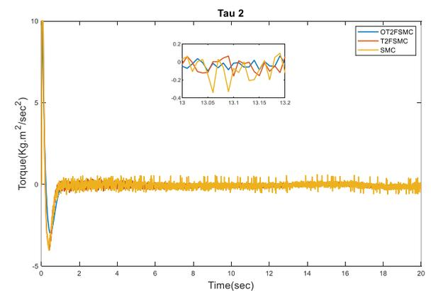
Fig. 16. Control signal of the link 2
