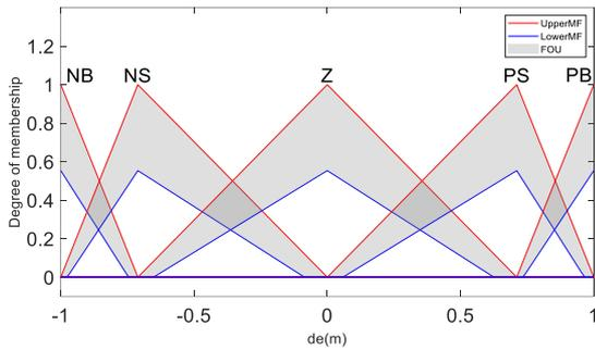
Fig. 10. The optimal membership function of rate of error
