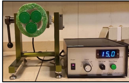
Fig. 2: Clinorotation of samples
