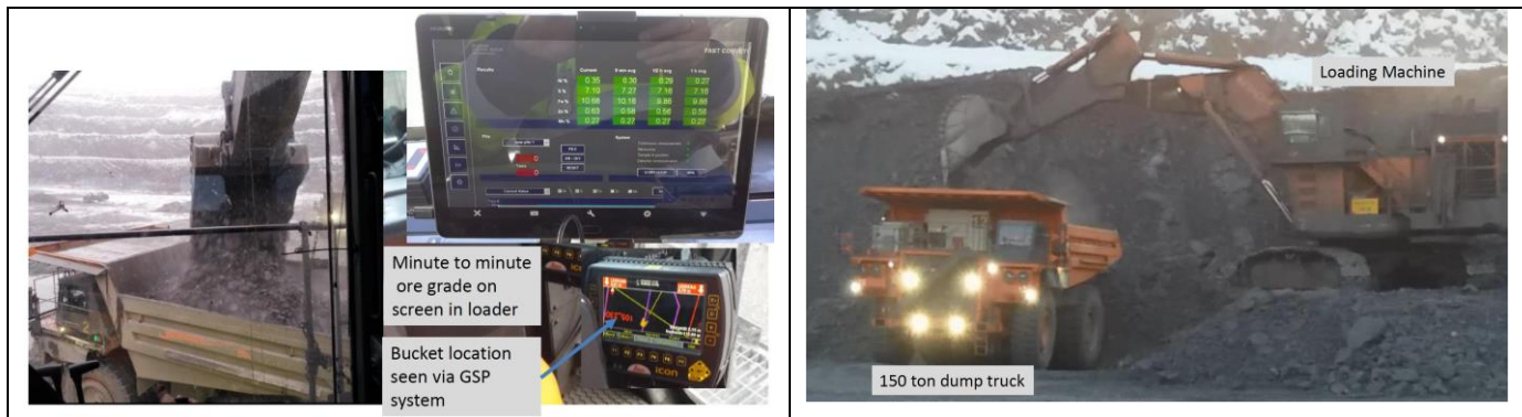
Fig. 4. An example of using data of the block model by driver of a loader. In the case of loading from unplanned area, the implemented alarm system allows correction of the loading operation [Courtesy of IMA Engineering].
