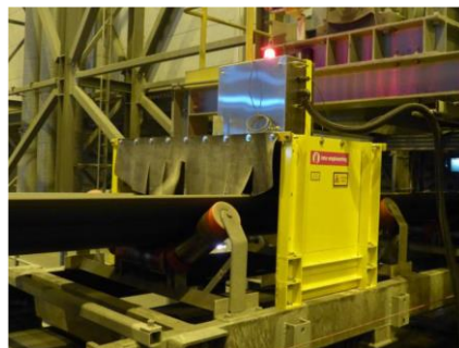
Fig. 5. Example of a smart XRF analyzer on conveyor belt. For smart grade control of the feed, the analyzer can be installed on the belts after the first and secondary crusher or during the processing stages [5].
