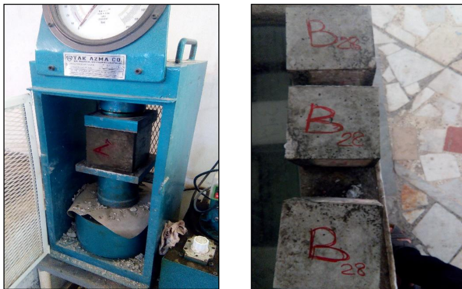
Fig. 4 - Compressive strength measuring device
