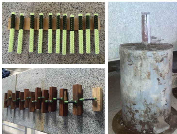
Fig. 1. Preparing of Pullout Specimens.
