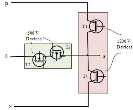
Figure 12 Bidirectional switch to the midpoint can be implemented with two IGBTs or GaN transistors
