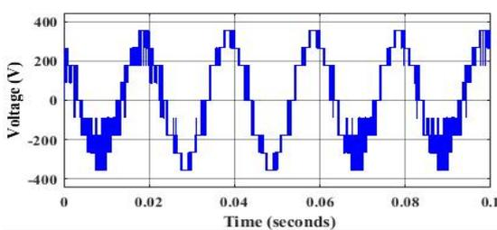
Figure 6 T-type output line to line voltage waveforms
