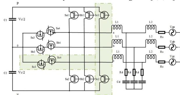
Figure 1 Three-level T-type inverter topology
