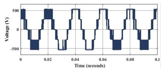
Figure 7 T-type output phase voltage waveforms
