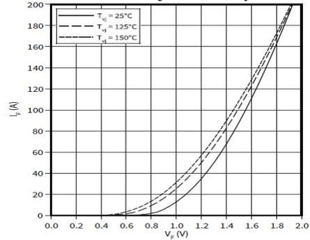
Figure 14 Measured forward voltage drop of the 1200V IGBTs for three different junction temperatures [25]
