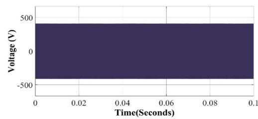
Figure 5 2L-NPC output phase voltage waveforms
