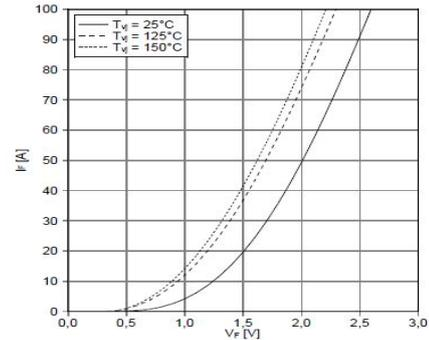
Figure 13 Measured forward voltage drop of the 600V IGBTs for three different junction temperatures [24]
