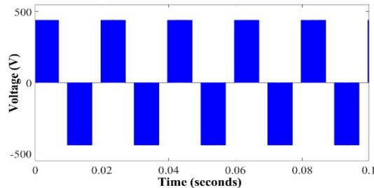
Figure 4 2L-NPC output line to line voltage waveforms
