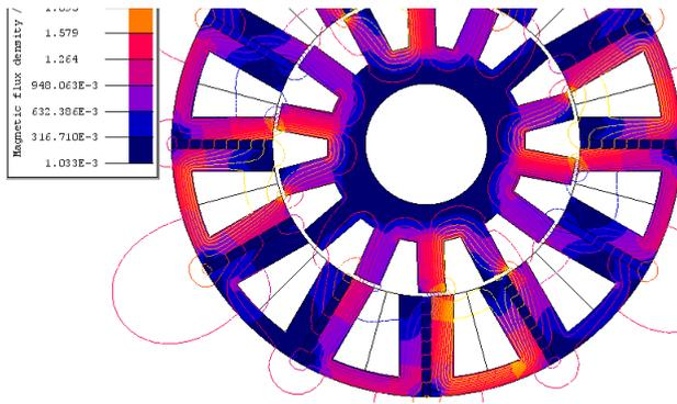
Figure 1. Distribution of magnetic flux density on the surface of the FSPM motor
