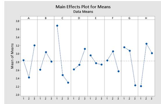
Figure 5. Main effects plot for the mean value of the torque ripple
