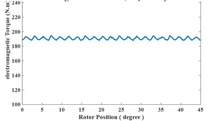
Figure 8. Electromagnetic torque of initial and modified
