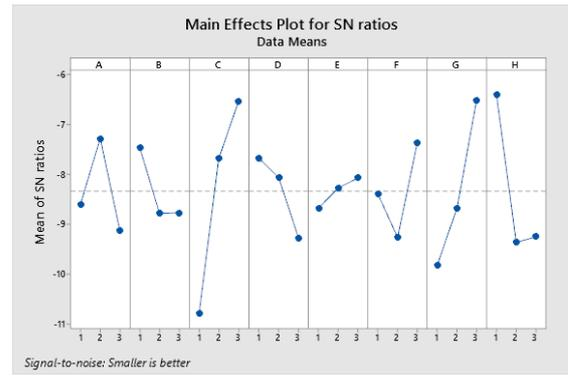
Figure 3. Main effects plot for S/N ratio of the torque ripple
