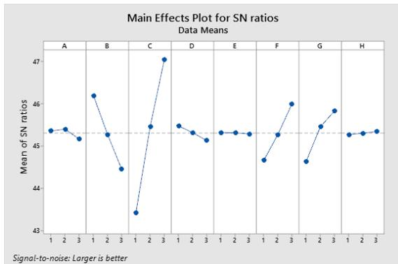
Figure 2. Main effects plot for S/N ratio of the torque
