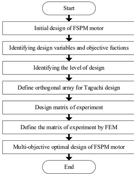
Figure 6. Taguchi optimal design procedure
