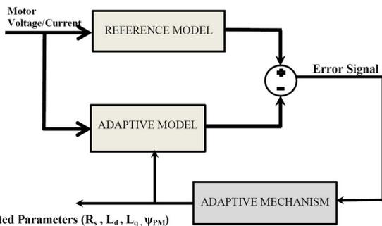
Figure 3. Schematic of the MRAS parameter estimation method
