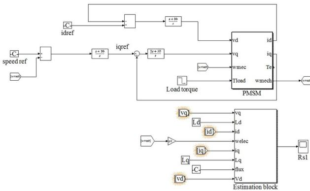
Figure 6. Overall system simulation scheme
