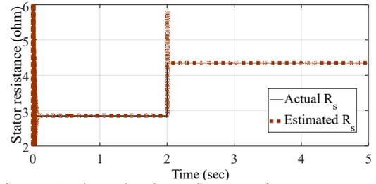
Figure 7. Estimated and actual stator resistances
