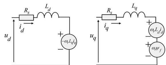
Figure 1. Equivalent d-q circuits of a PMSM
