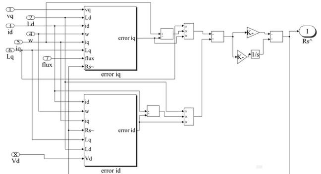
Figure 4. Stator resistance estimation scheme
