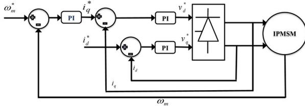
Figure 2. Block diagram of vector-controlled motor
