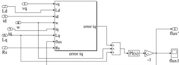
Figure 5. PM flux linkage estimation scheme
