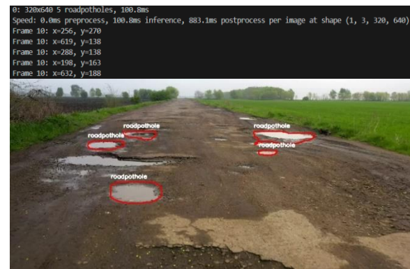
Fig 2. Simulation result for a frame of video with detected potholes
