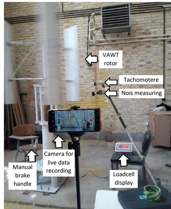
**Figure 7.** Measuring setup. A mobile phone camera is simply used to record live data from the loadcell display, tachometer and other sensors of the experiment.
