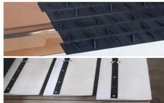
Figure 4. Top: Designed VG belt. Mid: Vortex generating pieces made by 3D printer. Down: Installation of the VGs the blades.
