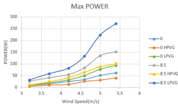
**Figure 11.** Maximum power at different speeds in the states without vortex generator, vortex generator on the high pressure side, vortex generator on the low pressure side
