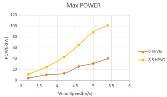
**Figure 9.** Maximum power versus wind speed at two pitch angles of 0 and 8.5 degrees, in the case of VGs installed on the high pressure side of the blade.
