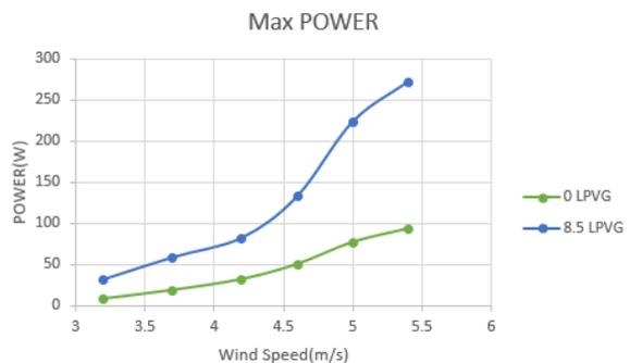
**Figure 10.** Maximum power versus wind speed at two pitch angles of 0 and 8.5 degrees, in the case of VGs installed on the low pressure side of the blade.
