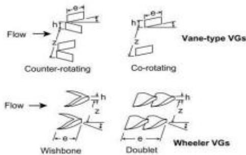
Figure 1. Types of vortex generators
