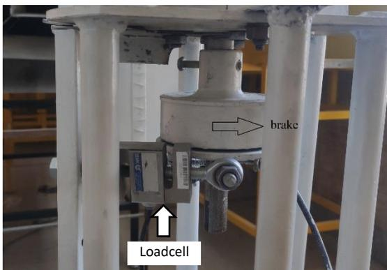
**Figure 6.** The workshop dynamometer including a frictional brake and a S-type loadcell measuring the rotational torque.
