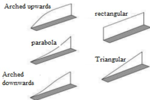
Figure 2. Types of blades of vortex generators
