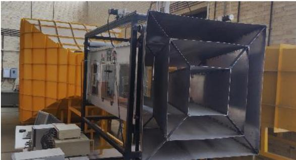
**Figure 5.** Wind tunnel equipped with a out-section diffuser available in the Energy Laboratory of Shahrood University of Technology
