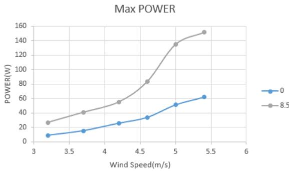
**Figure 8.** Maximum power production versus wind speed in the state without vortex generator at two pitch angles of 0 and 8.5 degrees
