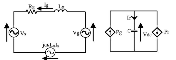
Fig. 5. Equivalent circuit for converters to analyse power
