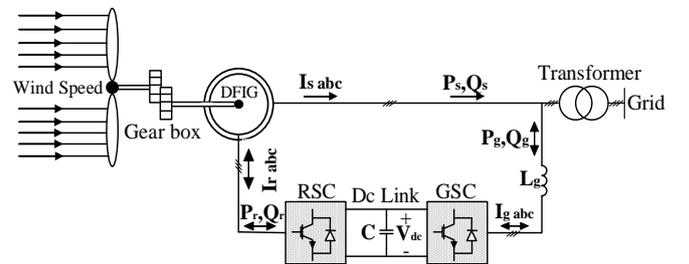
Fig. 1. DFIG with back-to-back converters
