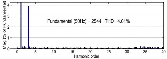
**Fig. 12.** Harmonic pollution of stator current before balanced stator current
