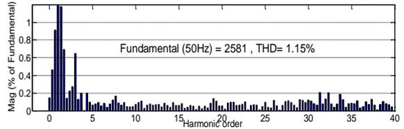
**Fig. 11.** Harmonic pollution of stator current during balanced stator current
