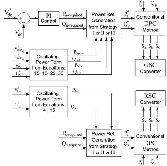
Fig 6: Block diagram of proposed method
