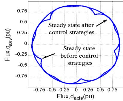
**Fig. 18.** Stator flux in dq axes in various control strategies
