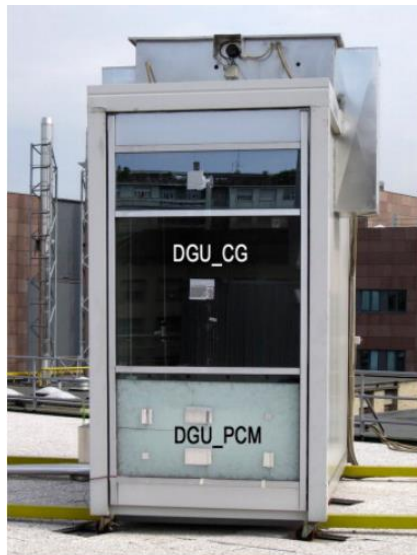
Figure 5, Test cells employed by Goia et al. [20], composing DGU clear glass and DGU-PCM
