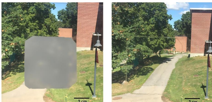
Figure 4, The solid-solid phase transition. Left: cold, crystalline, and opaque. Right: hot, amorphous, transparent [14]
