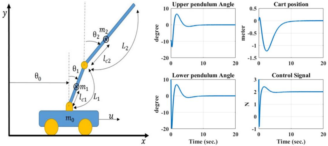
FIGURE 1. (Left) Conceptual Schematic of the DIPOAC, (Right) result of the simulations.
