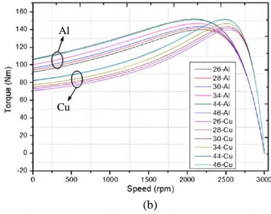
Fig. 5. Torque-speed characteristic curves a) single cage, b) double cage
