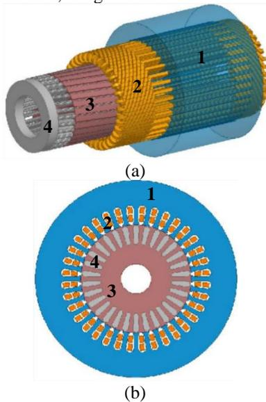
Figure 2. Model of Initial Design (1-Stator, 2-Winding, 3-Rotor, 4- Squirrel Cage): a) 2D, b) 3D
