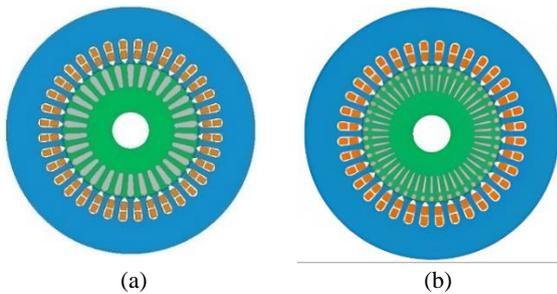
Fig. 6. Motor model a) initial design, b) optimized motor
