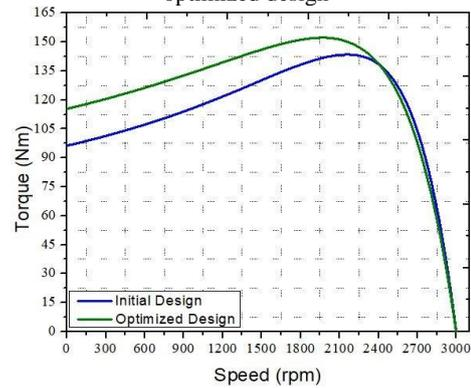
Fig. 8. Torque-speed characteristic curves
