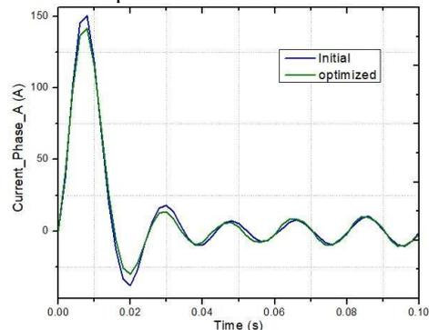
Fig. 9. Phase current waveforms of the motors in transient-state
