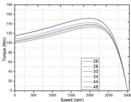
Fig. 4. Torque-speed characteristic curves in a double cage rotor
