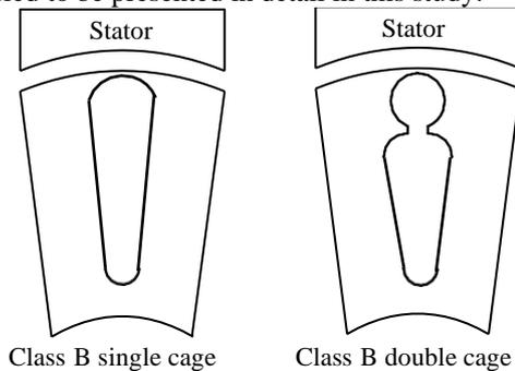
Figure 1. Slot structure
