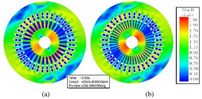
Fig. 7. Magnetic flux density distributions, a) initial design, b) optimized design
