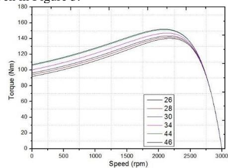
Fig. 3. Torque-speed characteristic curves in a single cage rotor
